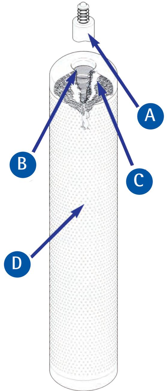
**A** Different end-configurations assure direct interchangeability with EMD, G.E., Alco and Bombardier locomotives.
