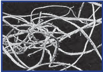
*Wood absorbs water and acids (extending lube oil drain intervals) and improves the filter's flow characteristics. Our wood is grown and processed here in Wisconsin, for excellent cost control.*
